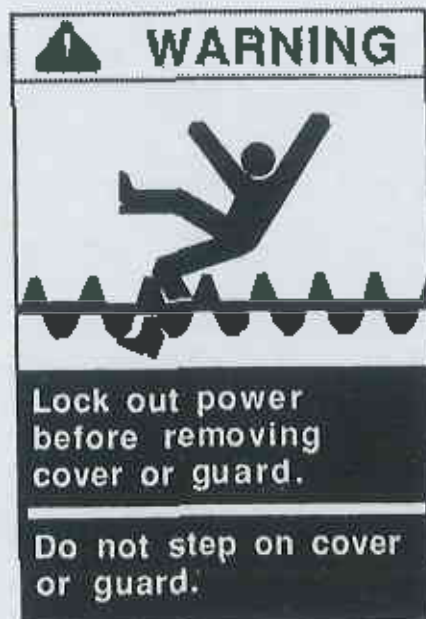
Figure 2-4 Warning Labels on the Screw Conveyor Belt Pulley Guard
