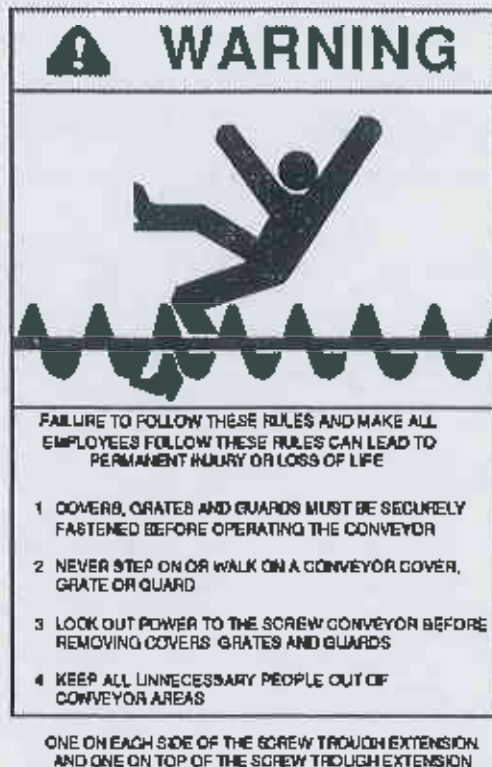
Figure 2-2 Warning Labels on the Screw Trough Extension
