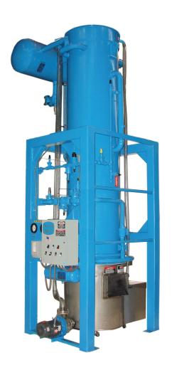
The P34AL Series with a capacity of 50 tons of ice per day is an ammonia low-side Tube-Ice machine designed to operate with a dedicated ammonia high-side or on a central refrigeration system. The P34AL will provide you with many years of dependable service.
