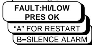
After the safety switch is reset it will be necessary to press the "A" button on the operator interface to return to the start up screen. Pressing "B" on the operator interface at this time will open the alarm contacts. Button "C" will always change the display to the set-up screen when a fault screen is displayed.
