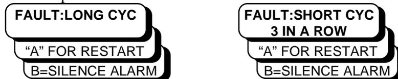
It will be necessary to press “A” on the operator interface to restart the machine.
